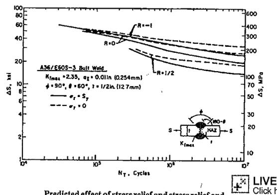
Predicted effect of stress relief and stress ratio on A36/E60S-3 butt weld fatigue life.
