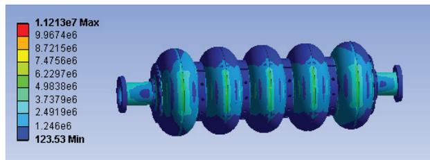
Figure 2: Equivalent stress of 5-cell cavity
