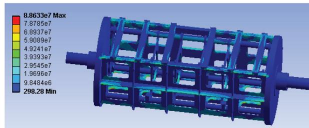
Figure 4: Equivalent stress of processing barrel.
