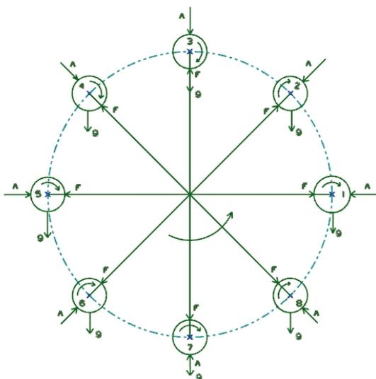
Figure 1: Schematic of eight load steps. g is standard earth gravity; A is centrifugal acceleration; F is media weight force.
