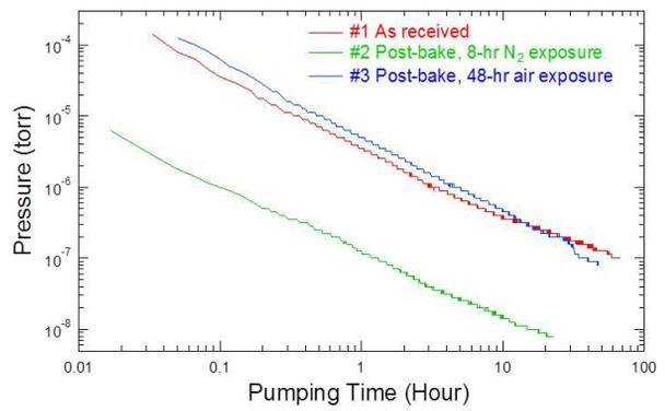
Figure 6: Pumpdown and outgassing test of the shrink-fit assembly. Besides the porous behaviour of the SiC no signs of gas burps from the shrink-fit could be observed.
