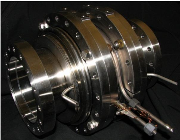
Figure 3: Picture of the HOM beamline absorber prior to installation in the HTC.
