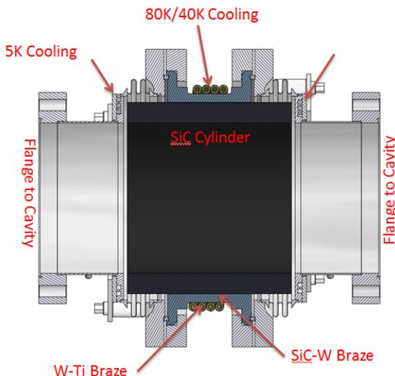
Figure 1: Cross-section of the HOM absorber currently being installed in the Horizontal Test Cryomodule (HTC). The absorbing material is SiC brazed to tungsten.
