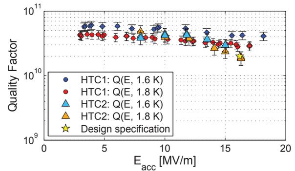
Figure 1: Quality factor measurements for HTC-1 and HTC-2 at 1.6 and 1.8 K after thermal cycling.
