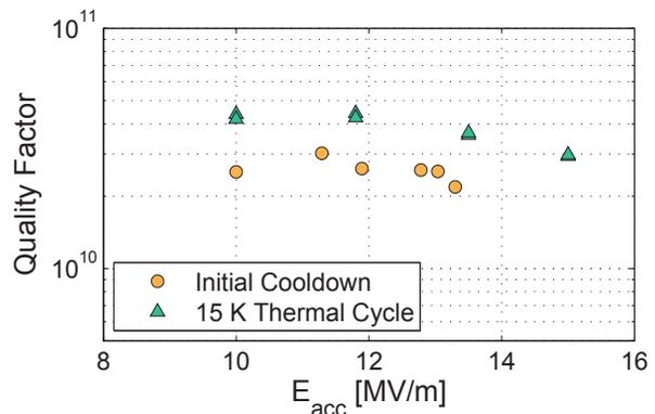
Figure 2: Quality factor in HTC-2 of the prototype cavity at 1.6 K measured before and after a 15 K thermal cycle. Vertical error bars (20%) have been suppressed for clarity.
