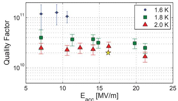
Figure 4: Initial Q vs E measurements for HTC-3. The star denotes the design specification for 1.8 K operation. The cavity field reached 21.2 MV/m, limited by available pumping capacity. Radiation at highest fields was  $< 1$  R/hr. The large uncertainties in the 1.6 K points arises from the small level of dissipated power, but are consistent with BCS predictions for a very low residual resistance cavity.
