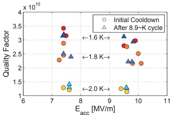
Figure 3: Quality factor in HTC-2 before (circles) and after (triangles) an 8.9 K thermal cycle. The colors correspond to data taken at the same temperature. There is no statistically significant change in mid-field Q in this measurement. Vertical error bars (20%) have been suppressed for visual clarity.
