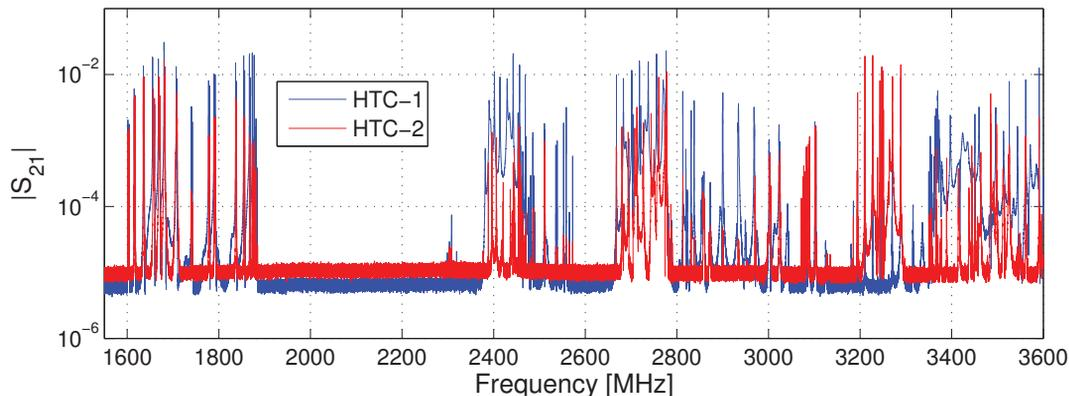
Figure 1: Amplitude of the scattering parameter  $S_{21}$  in the first two HTC experiments. The large quality factor of the modes are due to the fact that there were no HOM loads installed in HTC-1 and HTC-2. The mode frequencies agree with 2D simulations.
