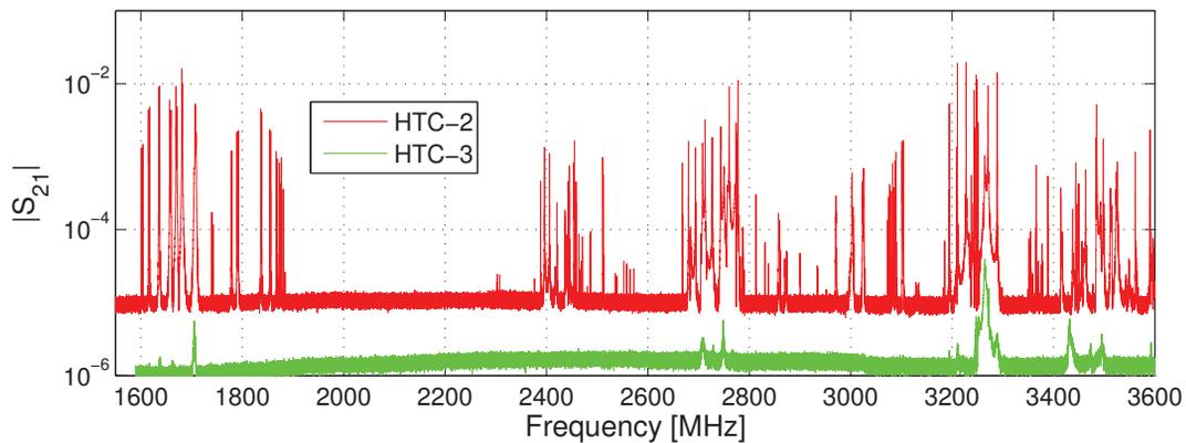
Figure 2: Amplitude of the scattering parameter  $S_{21}$  in the HTC-2 and HTC-3 experiments. The only significant change between the two runs is the beamline HOMs in HTC-3, showing strong damping of all modes.
