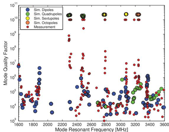
Figure 3: Reproduced from [10]. Comparison of simulated HOM spectrum and measured modes (red) in HTC-1. CLANS2 was used to compute dipole (blue), quadrupole (green), sextupole (yellow) and octopole (orange) modes from a 2D model. Error bars of 20% in quality factors have been suppressed for visual clarity. These Q's are high because of lack of HOM absorbers.
