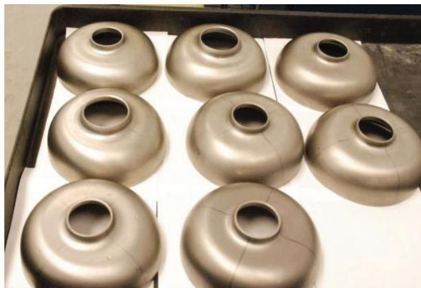
Figure 3: Formed niobium cups for the first LSF 9-cell prototype cavity.
