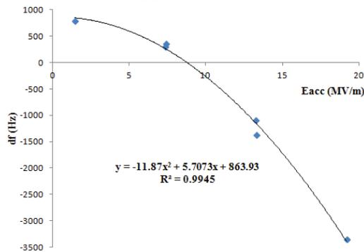
Figure 2: Lorentz detuning of the SRF gun cavity.
