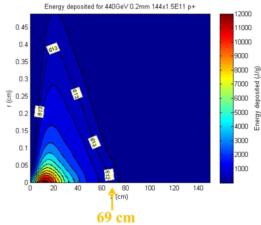
**Static simulations ONLY with FLUKA give a penetration distance of:
