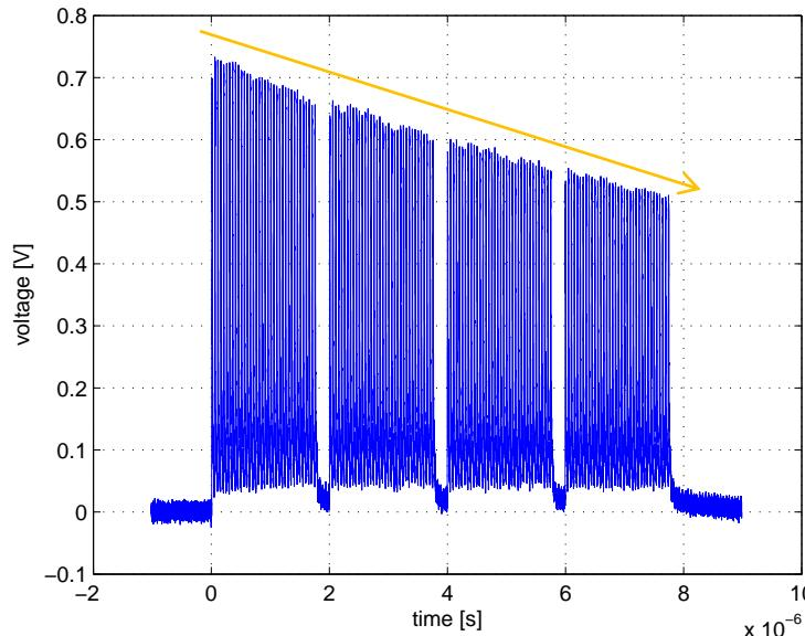
The signal from the first target is used to calculate the relation between voltage drop across the diamond with the decrease of efficiency.
