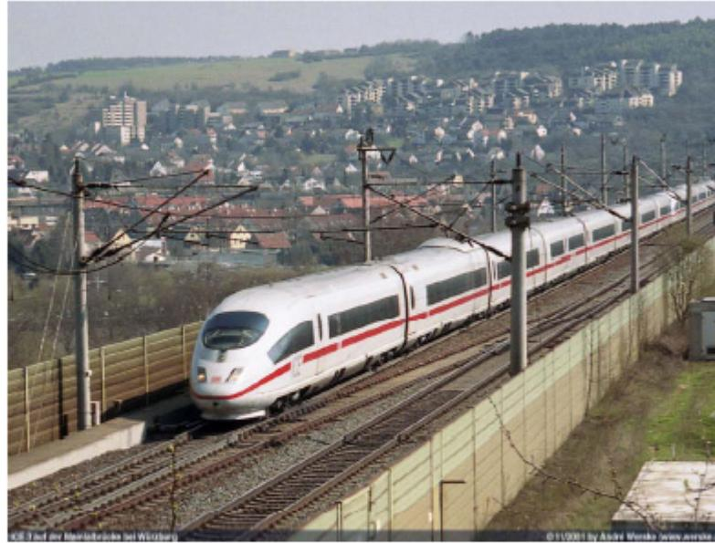
Kinetic Energy of a 200m train at 155 km/h  $\approx$  360 MJoule
