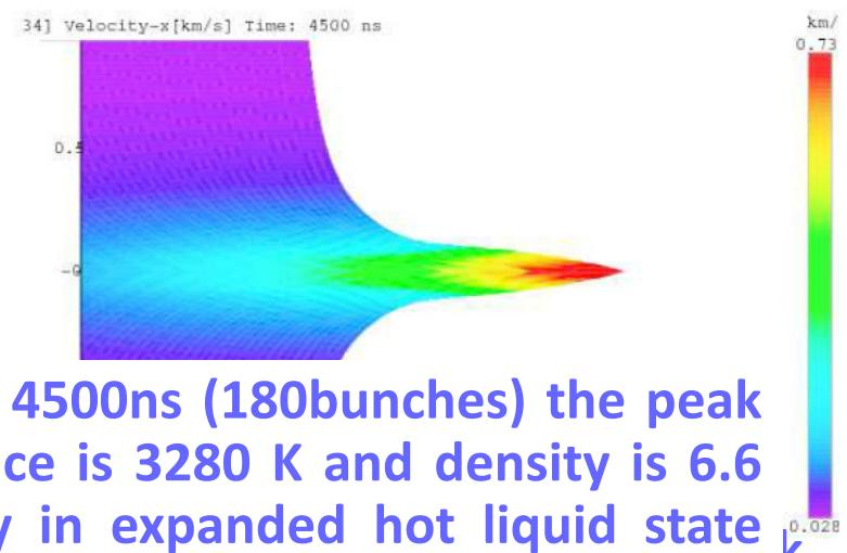
Simulation shows that after 4500ns (180bunches) the peak temperature on the front face is 3280 K and density is 6.6 g/cc, the material is mostly in expanded hot liquid state with little gas bubbles. The cohesion forces of the liquid will make it remain together. Any gas bubble will solidify in contact with the aluminum cylinder.
