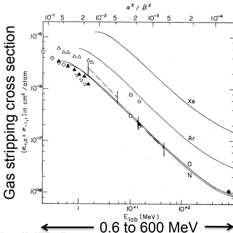
Cross section for double stripping ( $H^-$  to  $H^+$ ) is about 4% of cross section for single stripping ( $H^-$  to  $H^0$ )
