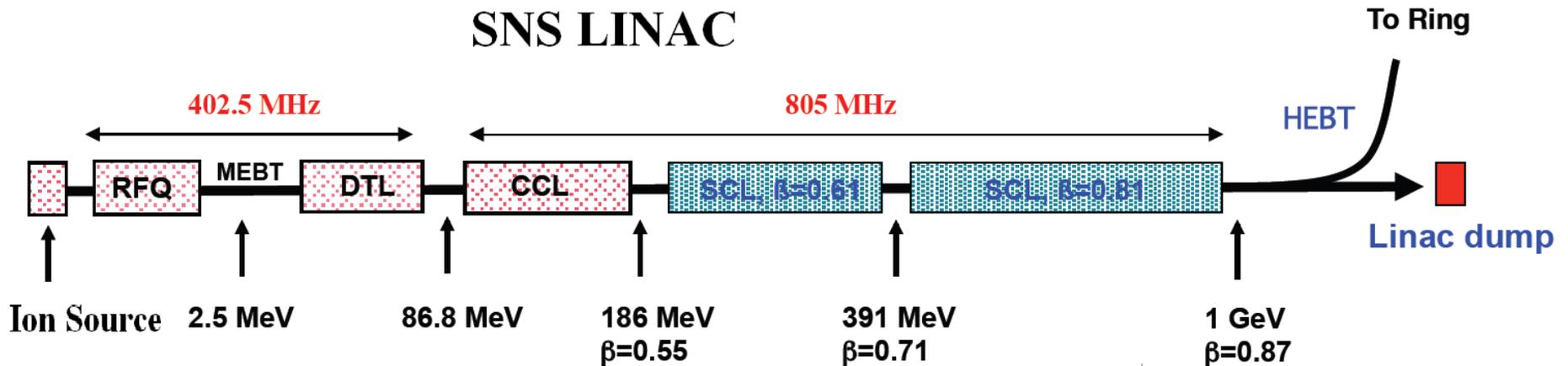
**Length: 330 m (Superconducting part 230 m)**
