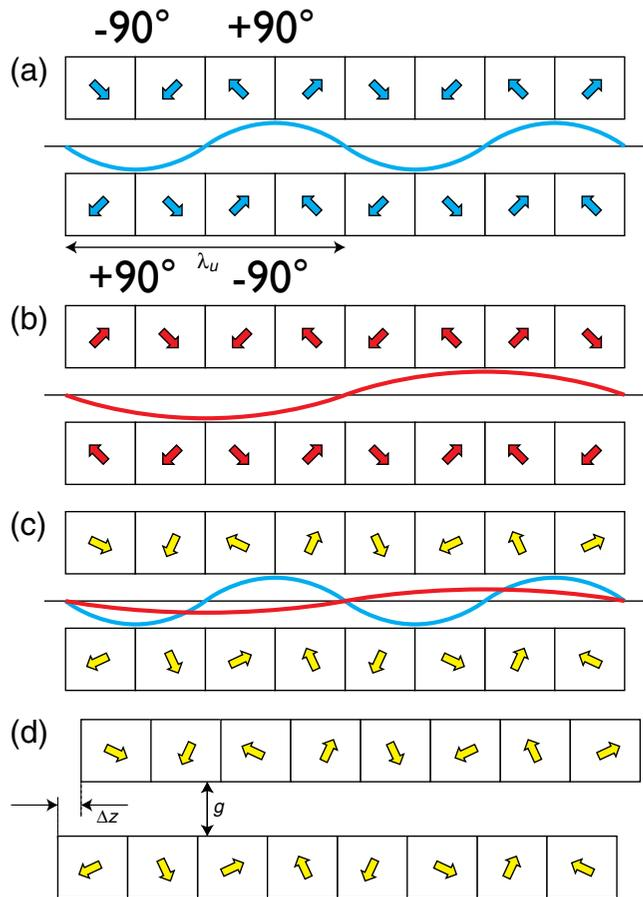
FIG. 1. Halbach-type undulator magnet circuits with four blocks per period (a) for the fundamental period and (b) for the double period. (c) Composite configuration of (a) and (b). (d) Two parameters to tune the photon energy: magnet gap  $g$  and magnet shift  $\Delta z$ .
