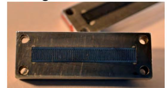
Laser-machined SmCo undulator array with 200- $\mu\text{m}$  thick, 2-mm long poles, 400- $\mu\text{m}$  period and 50 periods
