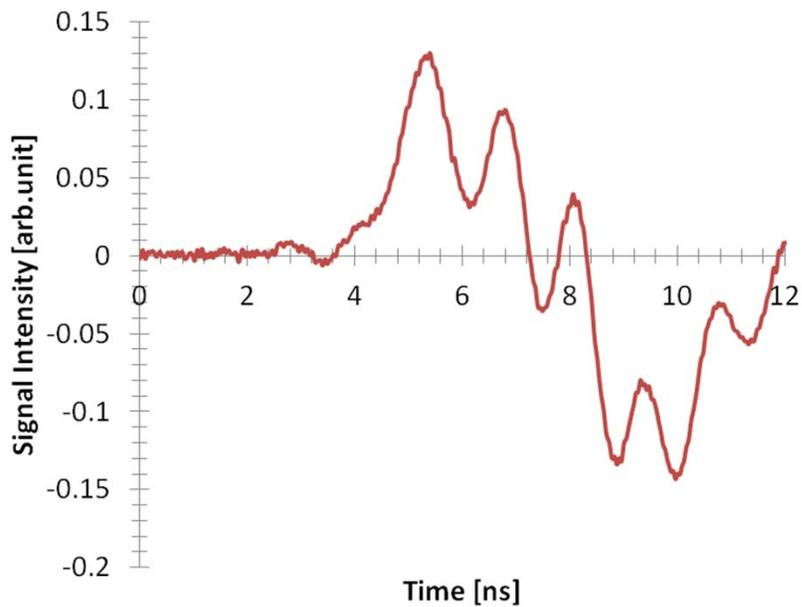
Capacitive probe raw signal.
