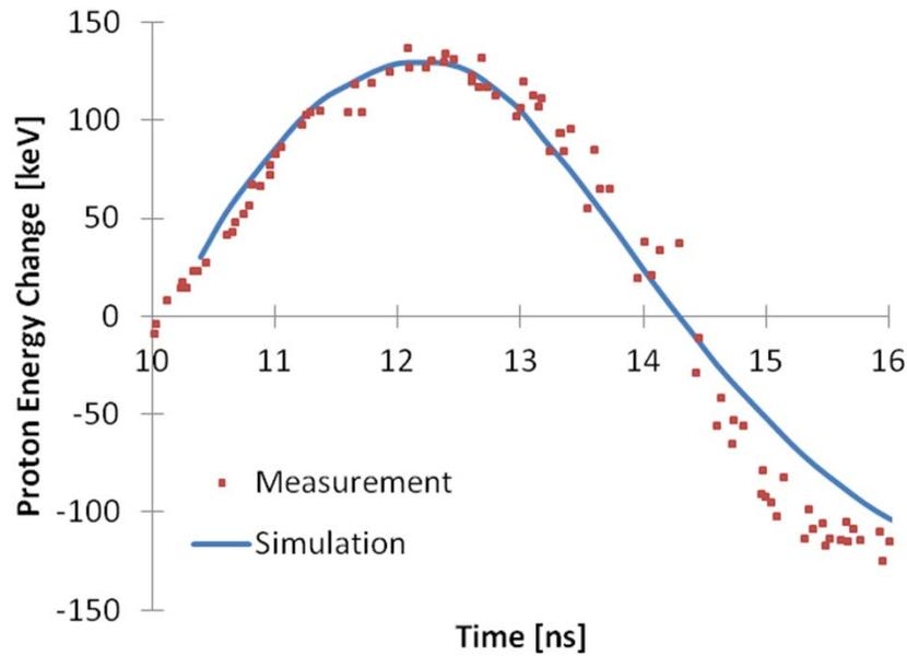
**Proton energy change at the exit of HGI for a ~10 kV charge voltage.**
