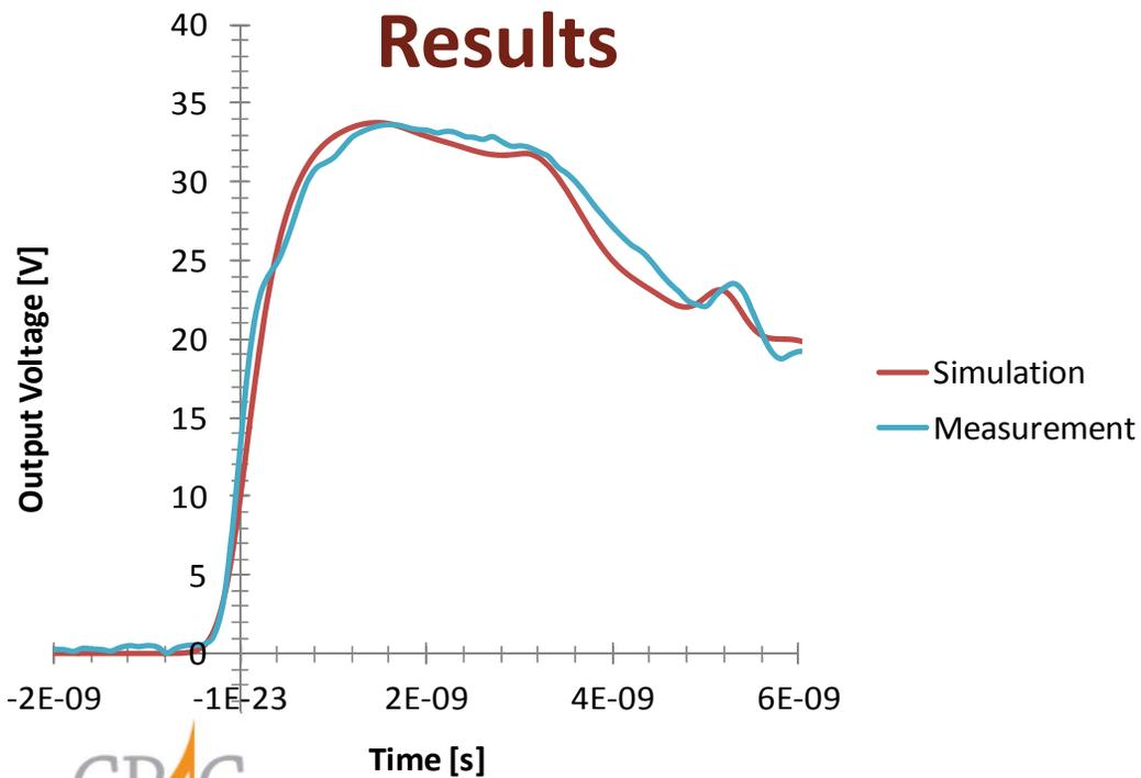
**Simulation agrees well with measured results in both magnitude and waveform.**
