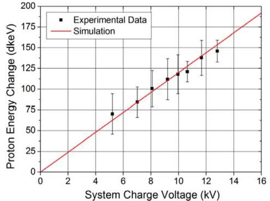
**Peak proton energy change for 5-13 kV capacitor charge voltage.**
