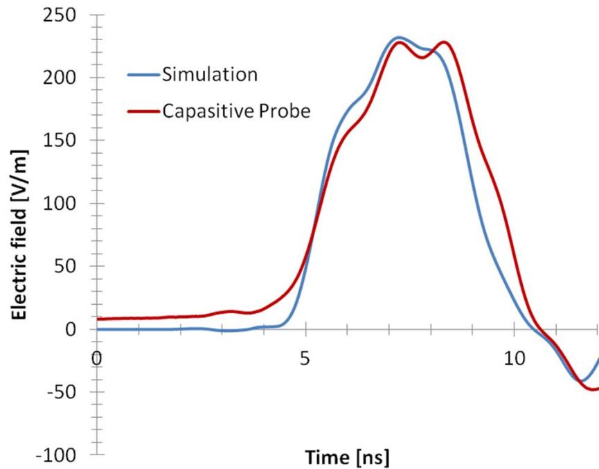
Simulated fringe field temporal profile and integrated capacitive probe signal.
