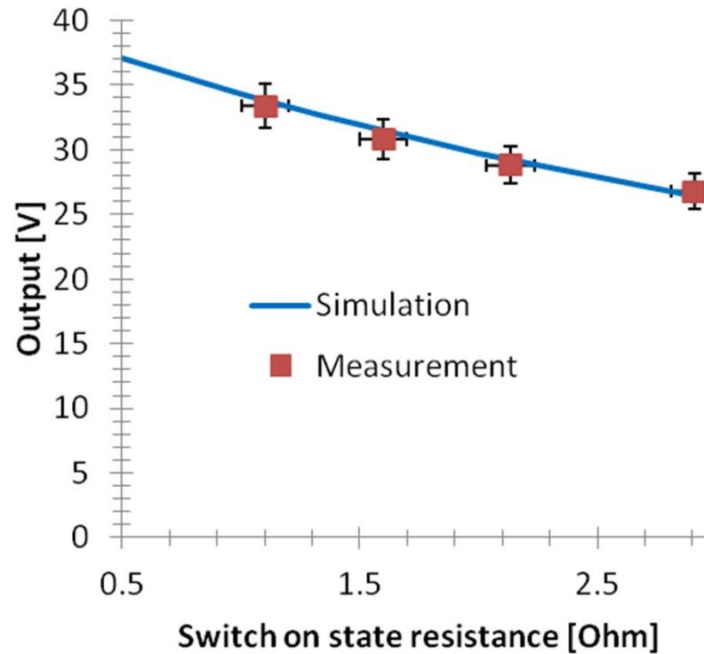
**Peak values of total output voltage measured at a low system charge voltage.**
