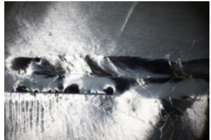
Optical inspection images of LR1-6, which quenched at 23 MV/m. Quench location on left.
