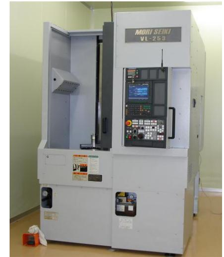
Vertical lathe for half-cell trimming
