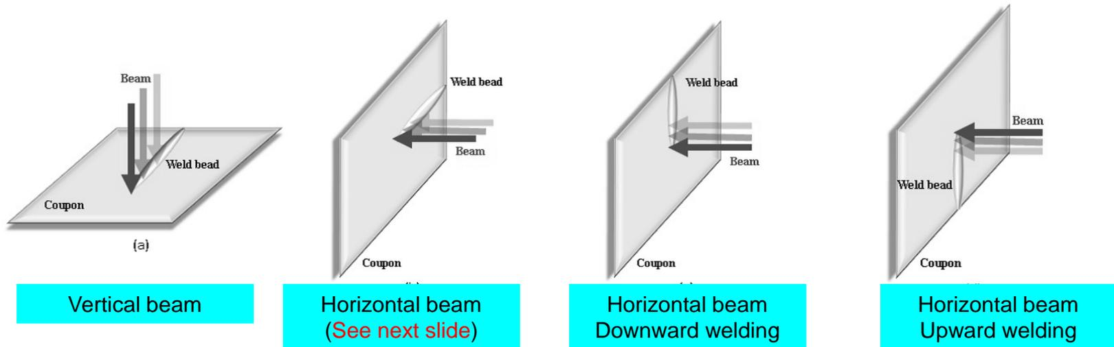
In particular, the gun and working-piece configuration affects the results of welding seam.
