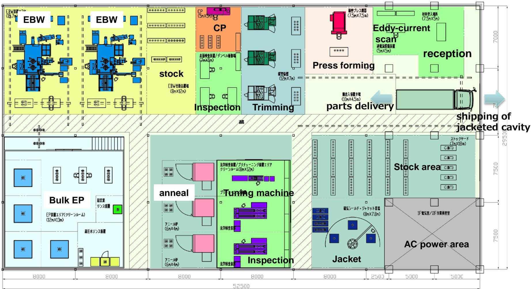
Assuming Nb plates for cell, fabricated end-group parts are input, 200 working days/year, 2 shifts/day with 30 people times 2 shifts
