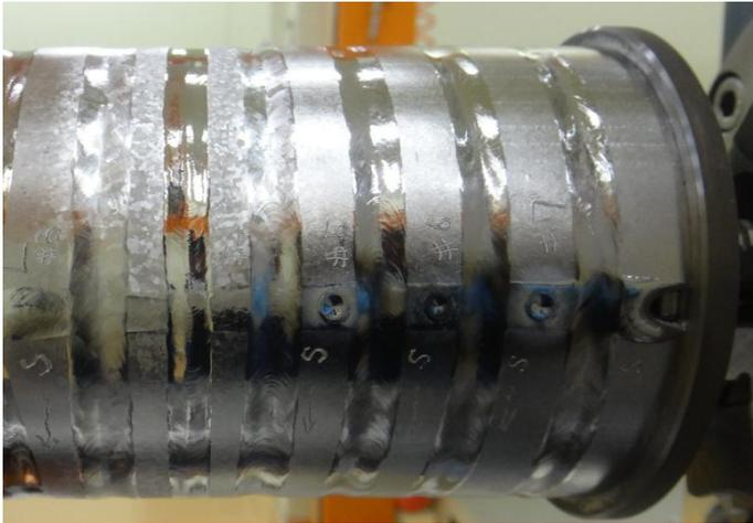
EBW test by a dummy Nb-pipe
