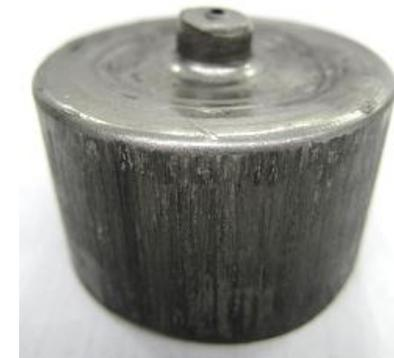
Trial to fabricate the freq. tuning tab by press-forming. (Under study)
