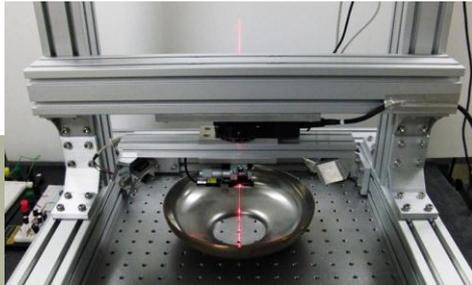
Measuring system for half-cell shape (Under developing)
