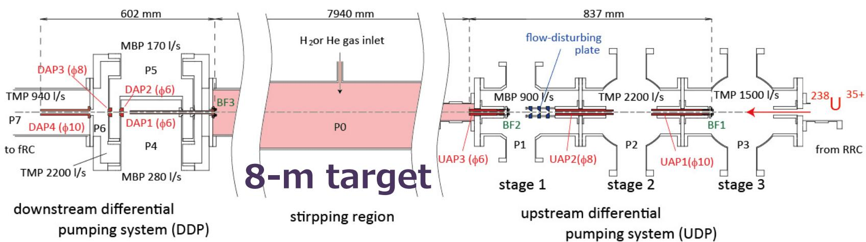
Gas was directly confined within **beamline** (H<sub>2</sub> 1 mg/cm<sup>2</sup>, He 3 mg/cm<sup>2</sup>)
