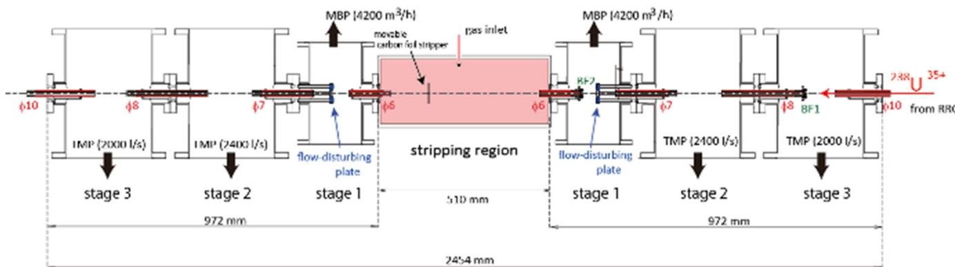
He gas w/ thickness of 2 mg/cm<sup>2</sup> was confined in **0.5-m target region**
