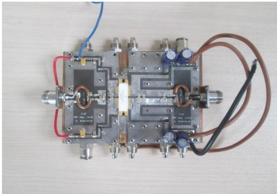
Amplifier module based on MRFE6VP61K25HR6 transistor
