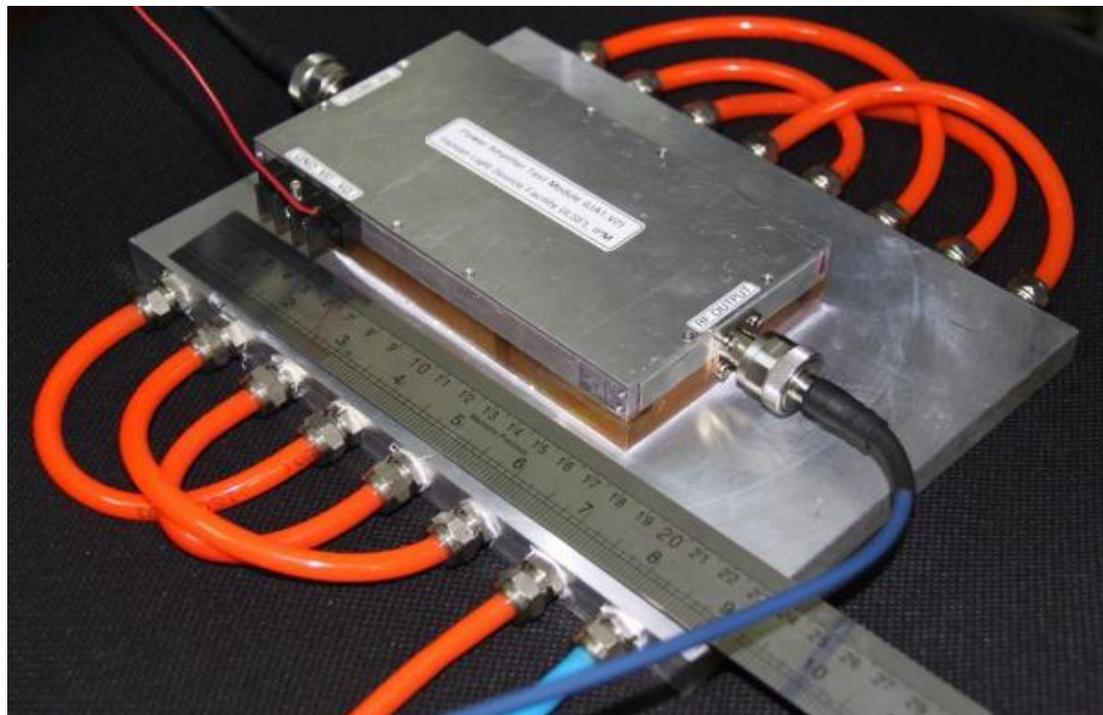
**Amplifier module based on BLF 578 transistor**
