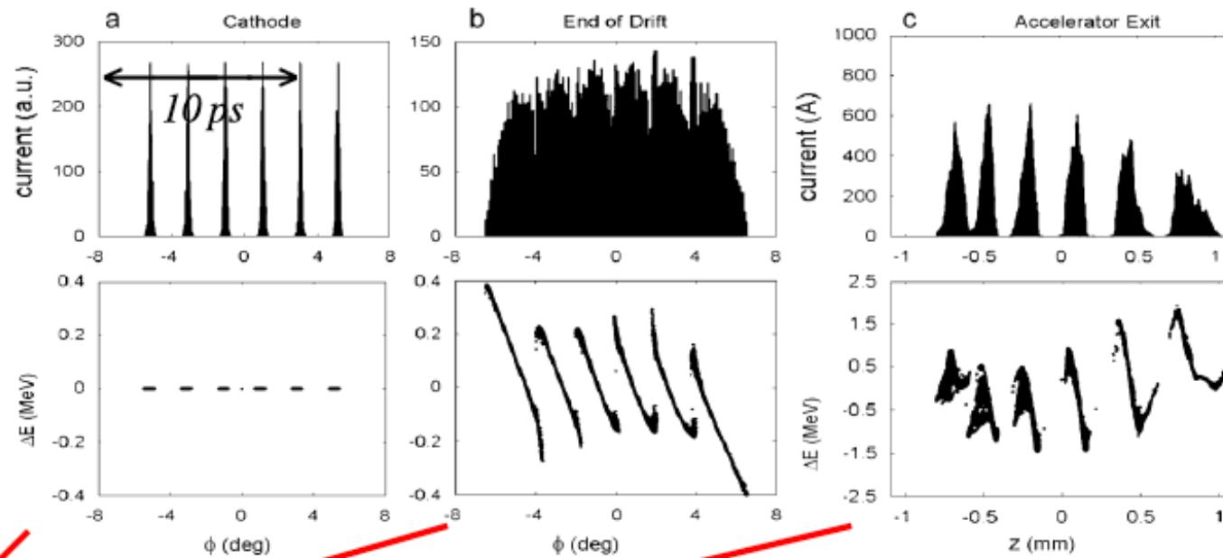
Fig. 1. Evolution of a six bunches electron beam train: the columns from left refers respectively to (a) the cathode, (b) the end of the drift at 150 cm and (c) the end of linac at 12 m far from cathode. The rows from top refer, respectively, to longitudinal profile and to energy modulation  $\Delta E$  (MeV).
