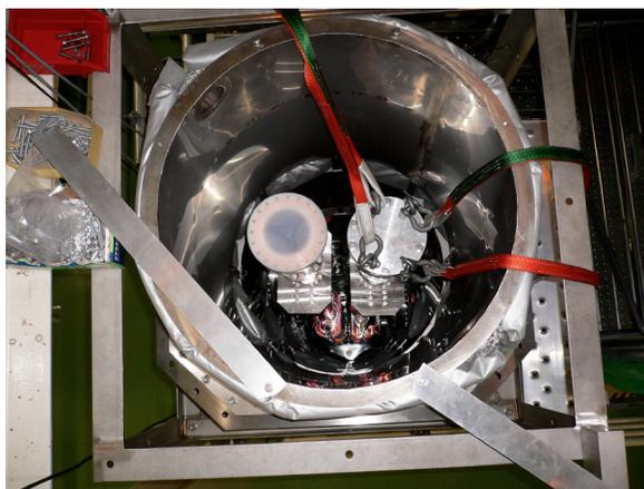
(upper): Inserting ante-chambers into a vertical TiN coating system. (lower): Top-side view of ante-chambers in two lines set in the coating system.
