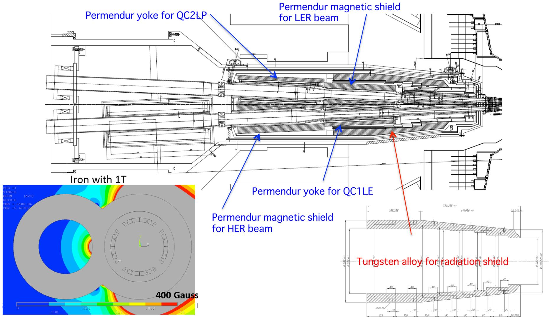
(2) To reduce leakage field on the other beam line, Permendur yokes and shields are adopted, instead of Iron.
