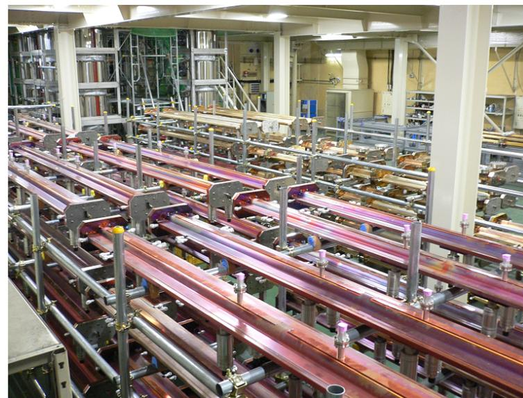
(upper and lower): Copper and Aluminum beam pipes after baking and TiN coating. They are temporary stocked in Oho B4 until moved to tunnel or other stock houses.
