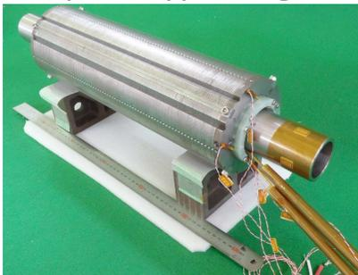
Successfully tested without any quench up to 2157A, well over the design current (1560A) for nominal operation.
