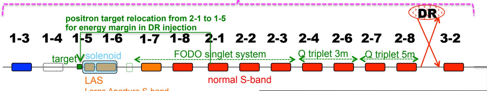
positron target relocation from 2-1 to 1-5 for energy margin in DR injection
