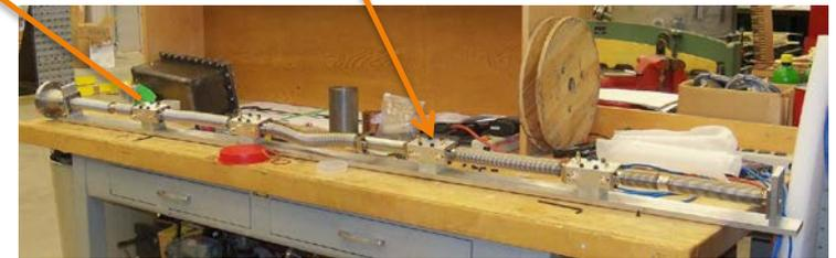
measured wire vibration frequency for the bench top set-up is 22.5 Hz
