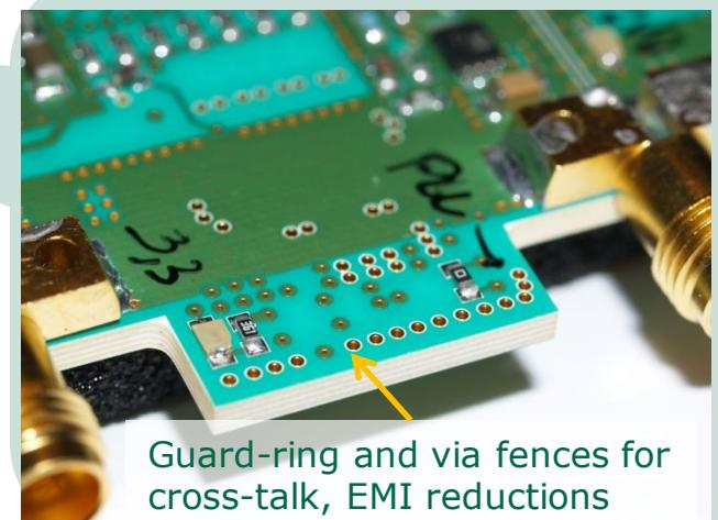
PCB made by ROGER 4003 consisting in 10 layers metal Stack-up
