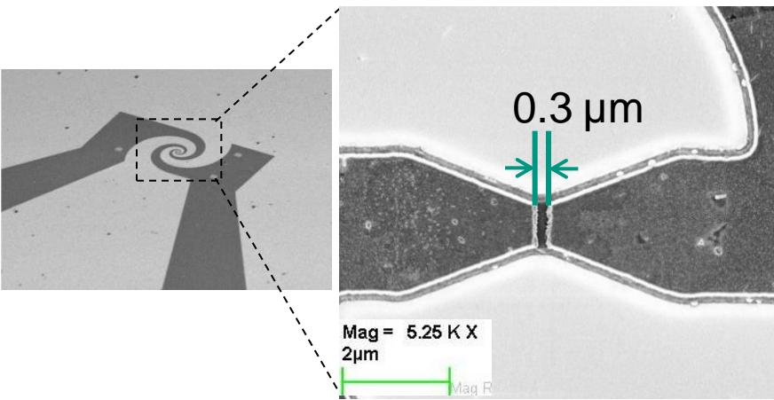
Nanometer-sized YBCO detectors in a high-speed readout system
