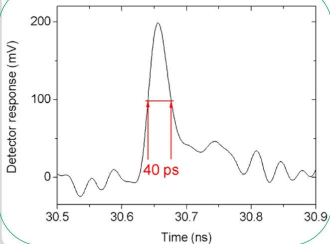
Detector system based on a superconducting NbN/YBCO ultra-fast bolometer with a bandwidth up to 1 THz.
