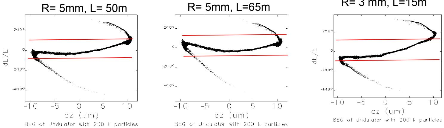
b) Corrugated pipe with radius of 3 mm,  $L=15$  m
