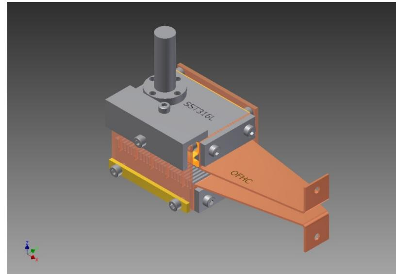
Adjustable gap type using two parallel plates with corrugations
