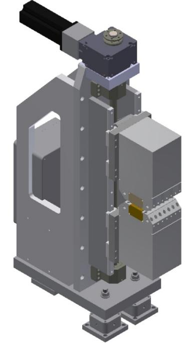
THPME027: Design and Fabrication of Prototype Phase Shifter for PAL XFEL
