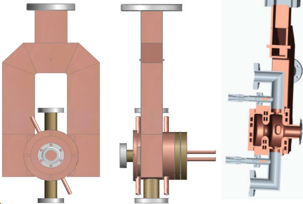
**PAL-XFEL baseline gun :** dual-coupler gun with additional two-holes to reduce quadrupole field
