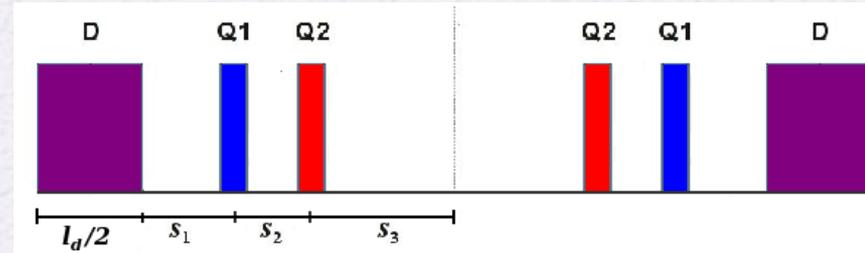
□ Analytical representation of TME quadrupole focal lengths (thin lens)
