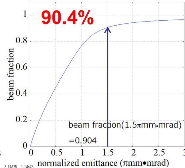
$\text{H}^-$  within the ellipse of  $\epsilon=1.5\pi\text{mm}\cdot\text{mrad}$  is calculated to be more than **60mA**.
