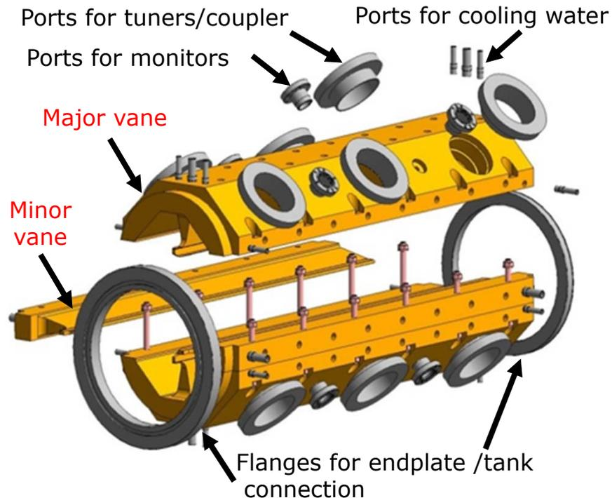
**Assembling of vanes and other components of the unit tank for brazing**
