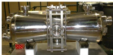
Figure 3: EM model of 162.5 MHz HWR (top), bare niobium cavity with stainless steel flanges (middle) and dressed HWR with slow tuner (bottom).
