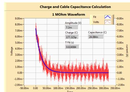
Figure 2: Wire charge measurement.
