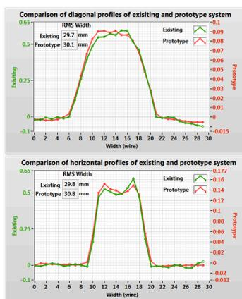
Figure 6: Profiles for a 5.7 uC proton beam.
