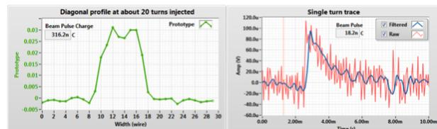
Figure 8: Low intensity profile and trace of a single turn beam.
