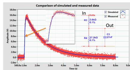
Figure 4: Analog circuit and measured signal.
