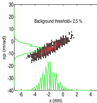
Figure 5: The horizontal emittance of RFQ is  $0.1203\pi\text{mm.mrad}$  measured with double slits system.
