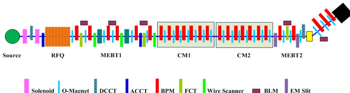
Figure 1: Beam instrumentation layout in C-ADS linac.
