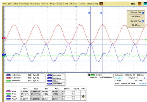
Figure 4: The beam energy of RFQ is 3.199MeV measured with two FCT with TOF.
