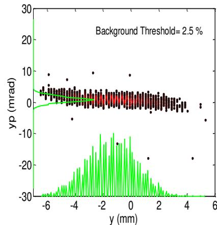
Figure 6: The vertical emittance of RFQ is  $0.1347\pi\text{mm.mrad}$  measured with double slits system.
