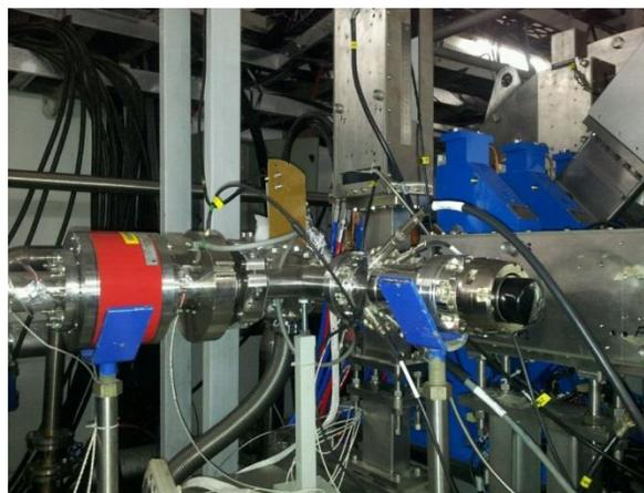
Figure 3: The electron beam scanner installed on the beam line for transverse beam profile measurement.
