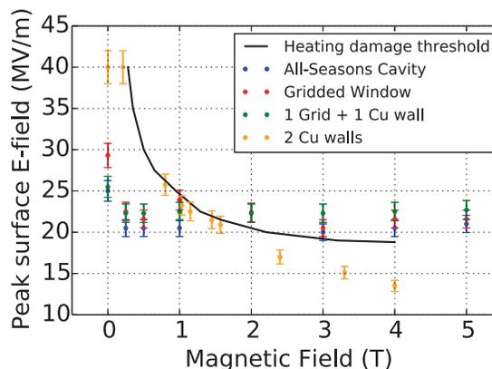
Figure 3: Peak surface electric field vs. external, applied  $B$ -field for cavity configurations described above. The black line indicates the threshold for surface fracture from beamlet heating, as discussed in [4].
