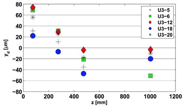
Figure 2: Displacements of the rotating coils axis with respect to the upstream magnets within five example U3 magnet blocks as a function of longitudinal position.
