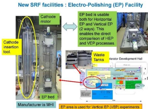
Figure 5: The current status of Electro-Polishing (EP) facility in COI buildings. EP bed and waste tanks were delivered.
