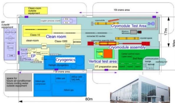
Figure 2: The layout plan of SRF facilities in the COI building.
