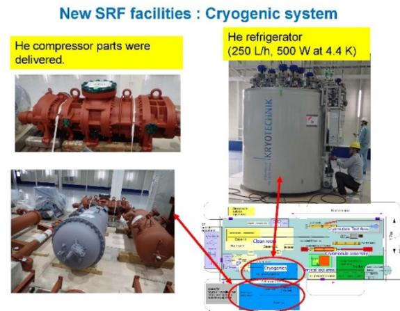
Figure 6: The current status of cryogenic system. The He refrigerator and He compressor parts were delivered.
