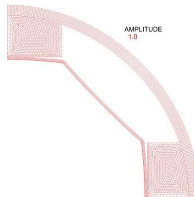
Figure 3: Deformation of the beam screen during a magnet quench.
