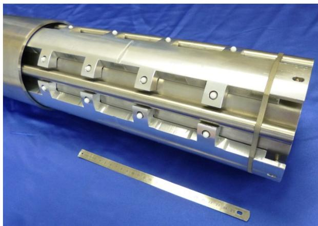
Figure 6: First beam screen prototype.
