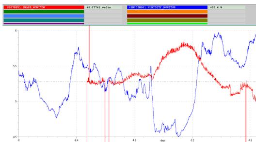
Figure 3: Stripchart of recorded humidity (Blue) and beam phase (Red) over several days (arbitrary units).
