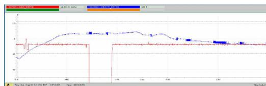
Figure 4: Stripchart of recorded humidity (Blue) and beam phase (Red) over several days (arbitrary units).
