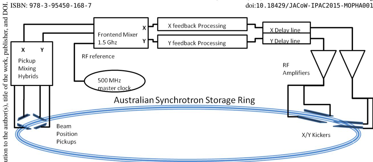
Figure 2: Overall layout of the transverse feedback system at the Australian Synchrotron
