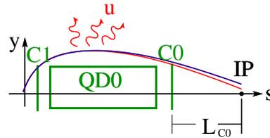
Figure 4: For the nominal trajectory in blue, the kick in C1 must cancel the kick in C0. For all particles that radiate in red, the difference in kicks should cancel  $\Delta y$ .
