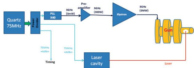
Figure 2: Drawing of PHIL RF chain and synchronization system.
