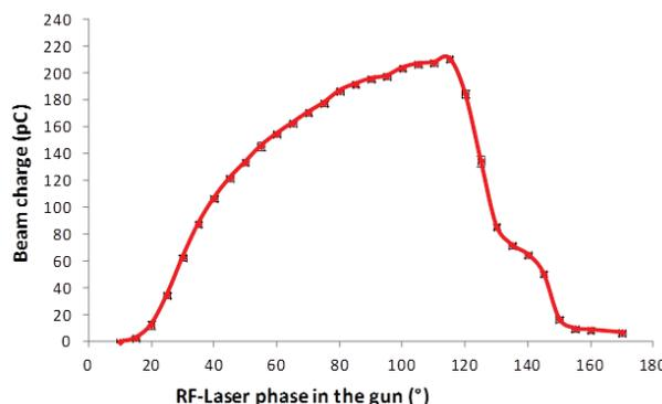
Figure 6: Beam charge Versus RF Phase.
