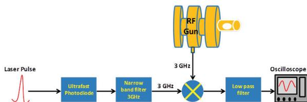
Figure 4: Bench measurement of the relative phase RF-Laser at PHIL.
