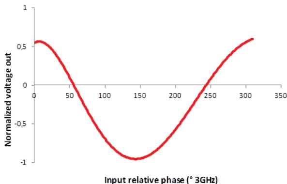
Figure 8: Transfer function of 3GHz mixer.
