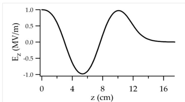
Figure 3: Normalized axial electric field of the RF photogun.
