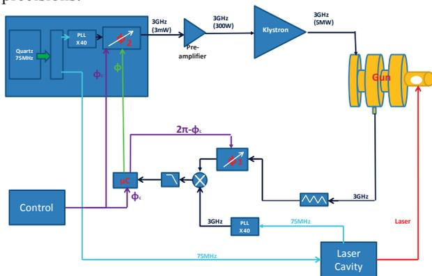
Figure 7: Schematic of feedback loop at PHIL.
