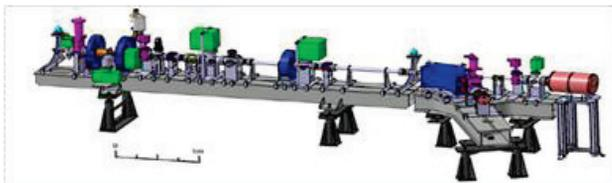
Figure 1: Drawing of PHIL beamlines. Blue boxes are magnetic elements; orange is the RF gun, green boxes stand for vacuum pumps.
