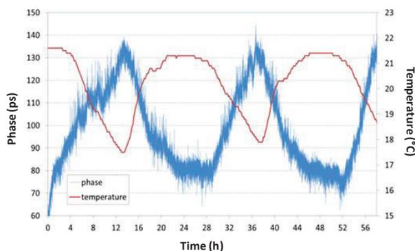
Figure 5: RF-Laser phase (blue) and temperature (brown) variations at PHIL.
