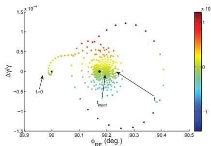
Figure 4: Synchrotron oscillation of a long bucket bunch and new stable solution after injection without tuning adjustment.
