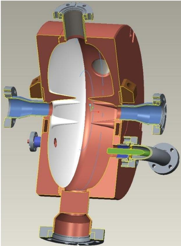
Figure 5: Final TCAV design for use in GunLab based on the second prototype [6].
