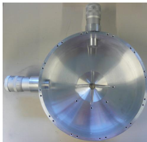
Figure 3: First aluminum prototype for low level RF-Tests based on the CAD design shown before.
