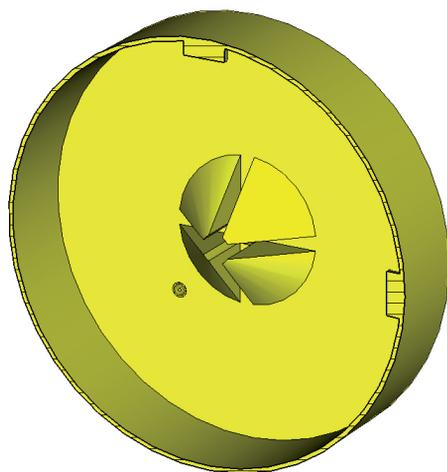
Figure 2: CAD design of our first TCAV prototype. Cylindrical shape with protrusions based on cones, two plungers and capacitive input coupler.
