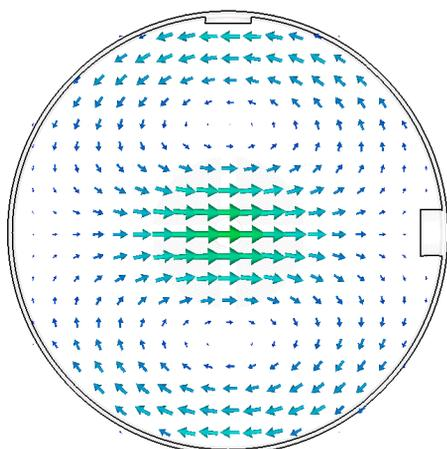
Figure 1: Magnetic field of a  $TM_{110}$ -like mode in the center of a cylindrical cavity. The plunger which protrudes deeper inside the resonator determines the polarization and by that the plane of transverse deflection.
