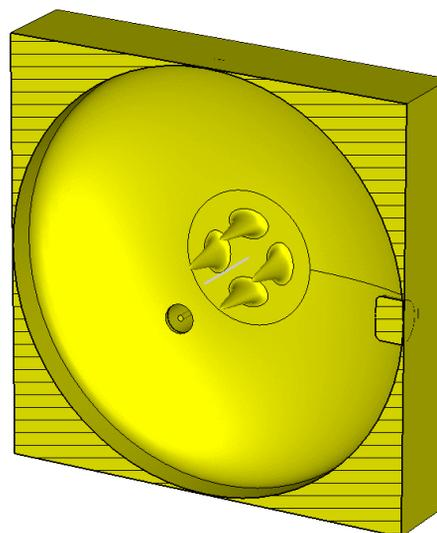
Figure 4: CAD design of our first TCAV prototype. Elliptical shape with protrusions based on sine function, two plungers and capacitive input coupler.
