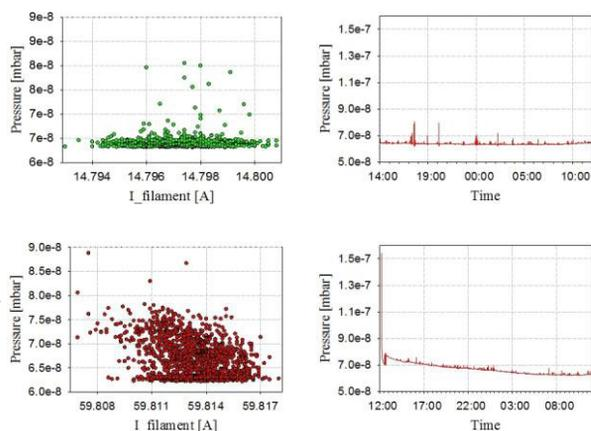
Figure 8: The de-gassing behaviour versus time at two different filament currents 15 A and 60 A.
