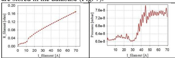
Figure 7: Filament resistance and chamber pressure vs filament current.
