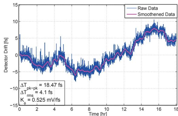
Figure 6: MZM based phase detector timing drift stability.
