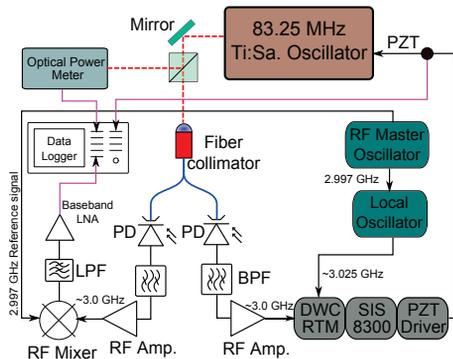
Figure 2: Detailed block diagram of DWC based locking setup with out-of-loop phase detector.
