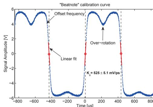
Figure 5: Calibration curve recorded by Oscilloscope.
