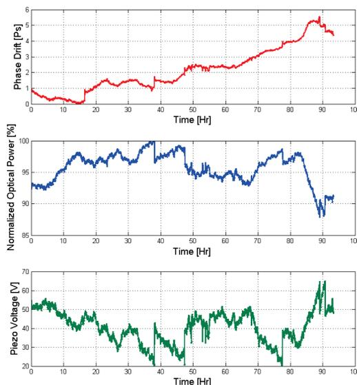
Figure 3: Measurement of long term out-of-loop phase stability, optical power and piezo voltage.
