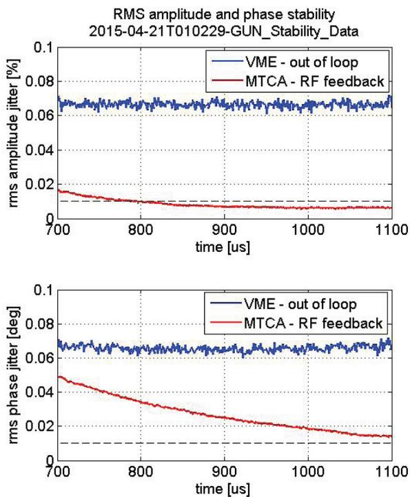
Figure 2: RF field stability (rms) of the FLASH gun during the flattop in amplitude and phase, averaged over 1 min.
