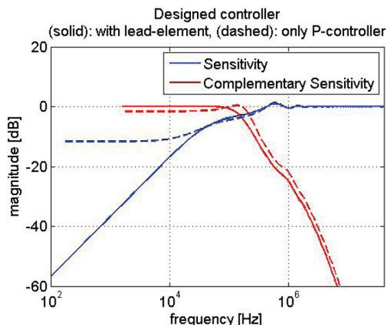
Figure 1: Sensitivity (S) and complementary sensitivity (T) function of the designed controller for the FLASH gun with lead-lag element (solid) and P-controller (dashed).
