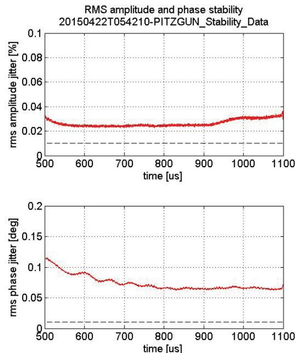
Figure 4: RF field stability (rms) of the PITZ gun during the flattop in amplitude and phase, measured over 5 min.
