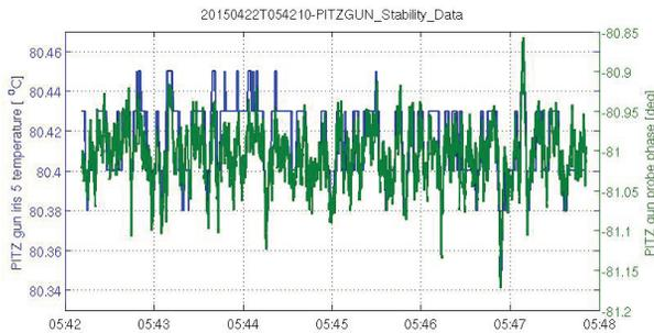
Figure 5: Gun probe phase and iris temperature (sensor Iris 5) at the PITZ gun.
