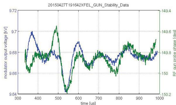
Figure 3: Modulator high voltage and gun probe phase during the flattop at the XFEL gun.
