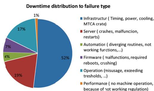
Figure 3: Statistic overview for MicroTCA installation and corresponding issues.
