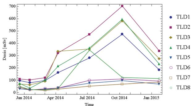
Figure 5: History of doses measured with TLDs at ACC1/39 (TLD1 to TLD4) and ACC23 (TLD5 to TLD8).
