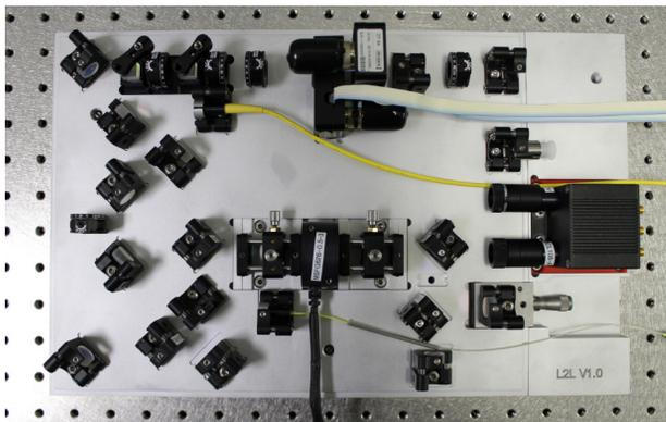
Figure 3: New engineered laser-to-laser synchronization setup. Outer dimensions: 375 mm x 235 mm.
