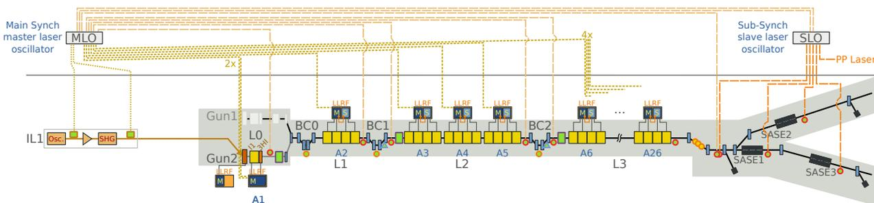
Figure 2: Schematic of the laser-based synchronization system at XFEL.
