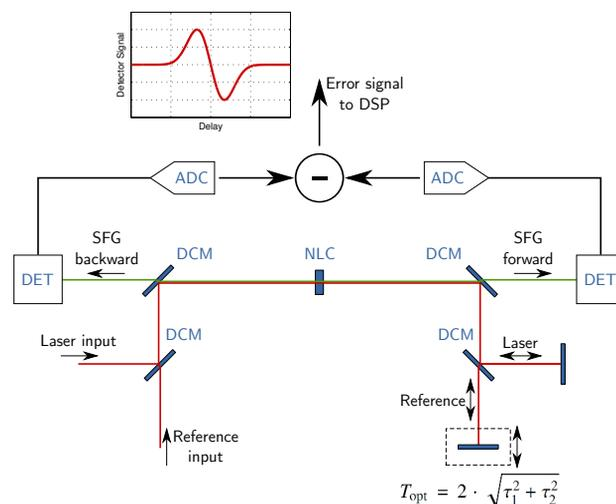
Figure 1: Principle of the balanced optical cross-correlator.
