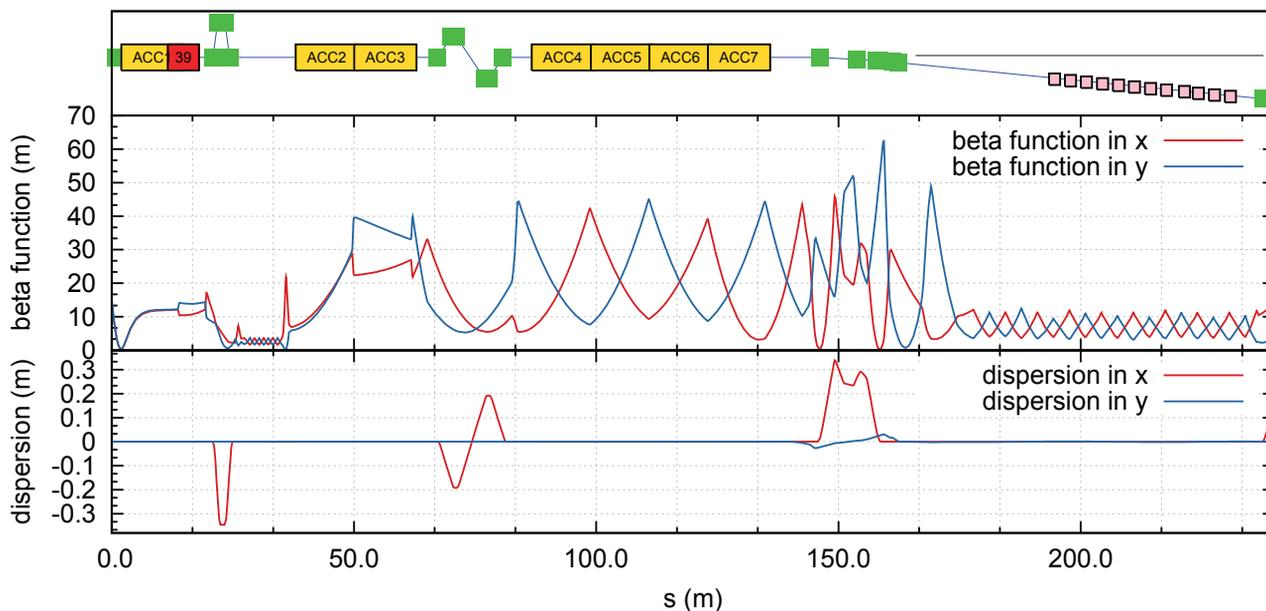
Figure 1: The FLASH2 design beta functions and the corresponding dispersion in both planes. Both plots show all sections of the electron beamline including the injector, the linac, the extraction arc, a matching section as well as the undulator.
