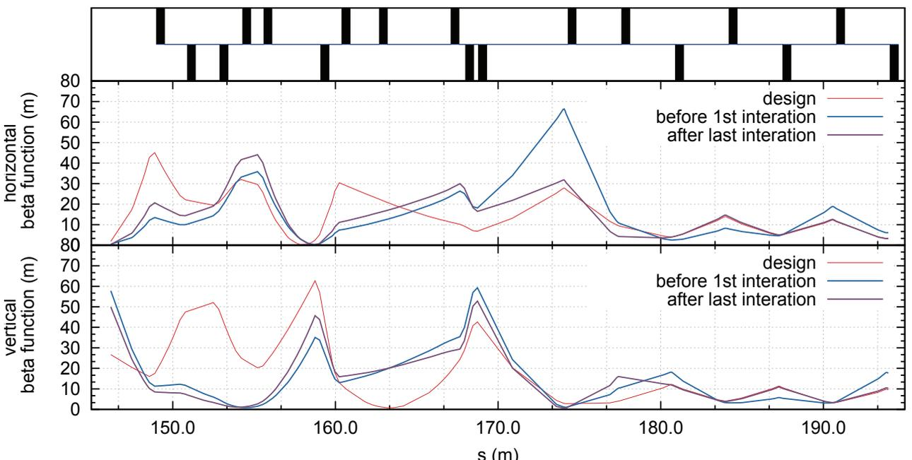
Figure 3: The horizontal and vertical beta function in the FLASH2 extraction arc and in the following matching section. The upper plot shows the horizontal plane and the lower plot the vertical. The red lines describe the design beta functions, the blue lines the reconstructed beta functions after the first optimization iteration and the purple lines represent the functions after the optimization was completed.
