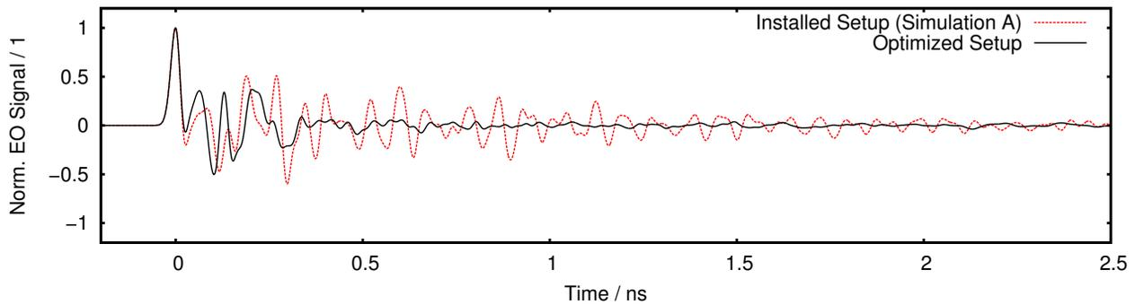
Figure 4: Simulated signal of the optimized and the currently installed EO setup (*Simulation A* from Fig. 2). Especially note the decrease of the remaining wakefield at  $t \approx 2$  ns, where a trailing bunch would be located.
