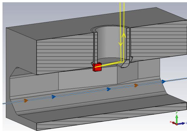
Figure 3: Cut through the beam pipe and the optimized EO setup. The electron beam and the laser travel similar to the one in Fig. 1. The mirror is now integrated into the arm, while the opening has been enlarged to allow the wake energy to leave the measurement area.
