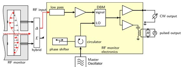
Figure 4: Illustration of the RF monitor electronics. The beam excites the fundamental mode of the resonator at 2.45 GHz. This RF power is converted to a voltage which can be monitored for CW beam or for pulsed beam.
