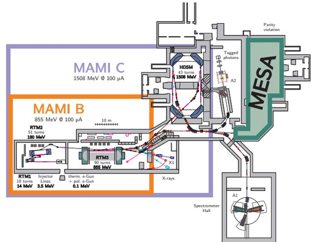
Figure 2: Floor plan of the MAMI accelerator. The space for MESA currently available is marked in green. The test setup at MAMI is installed next to the RTM3 where the beam has an energy of 180 MeV – similar to the external mode with 155 MeV of MESA.
