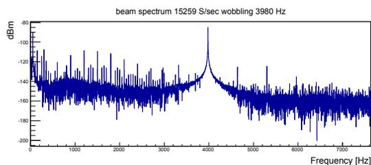
Figure 7: FFT extracted from the run control data while the beam is wobbled with 3980 Hz.
