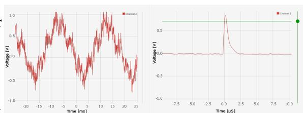
Figure 6: Signals RF monitors: Left side shows 8  $\mu$ A CW with its characteristic 50 Hz ripple, right side shows a diagnostic pulse of 10 ns being lengthened by the limited bandwidth of the analog electronics. Both shots were performed with the original FPGA firmware.
