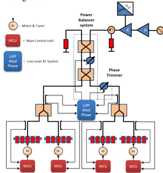
Figure 6 : Control Loops of first LLRF module.
