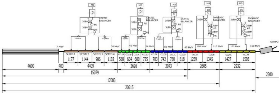
Figure 1: Block scheme of TOP-IMPLART RF system.
