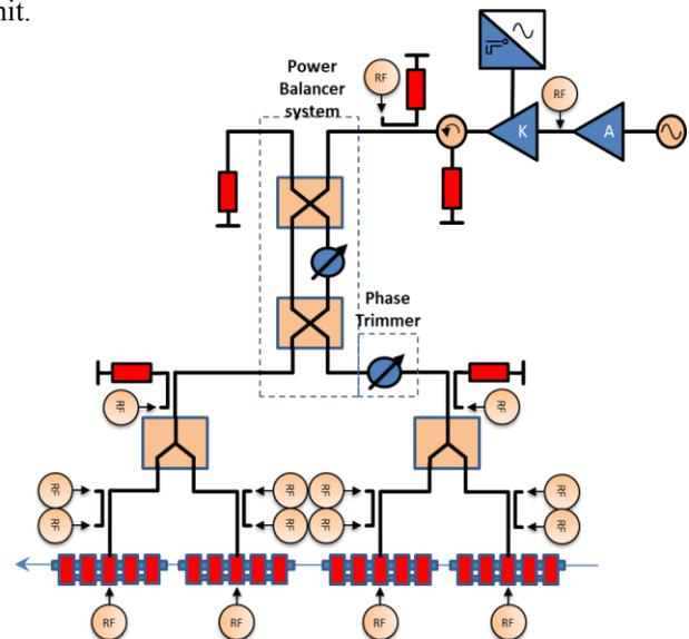
Figure 3: RF distribution to SCDTL structures.
