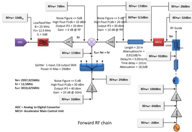
Figure 4: Signal conditioning and frequency down-conversion of the forward RF signal.
