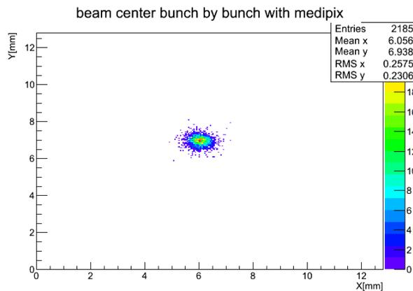
Figure 6: XY plot of the beam centroid position for 3500 bunches of 450 MeV electrons.
