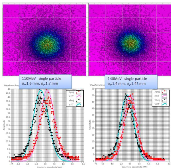
Figure 5: Run-time beam stability for different energy settings, maintaining the single particle multiplicity (with some tuning to match users' needs).
