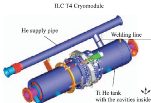
Figure 1: He-vessel connect to He-supply pipe.
