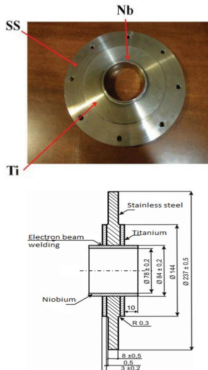
Figure 4: Nb+Ti+SS sample.
