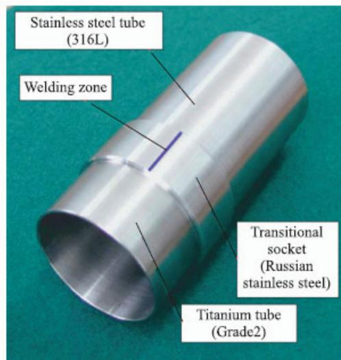
Figure 2: Ti+SS transition element.
