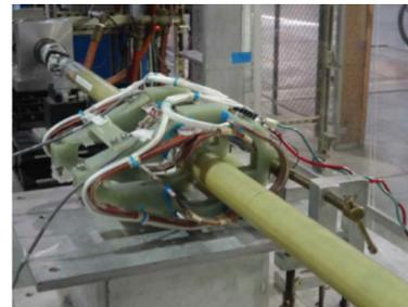
Figure 4: Ante-chamber type dithering coil is being measured by a rotating system.
