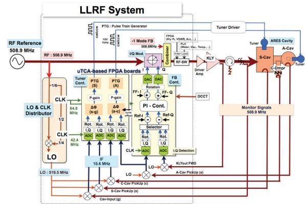
Figure 1: Block diagram for ARES cavity control.
