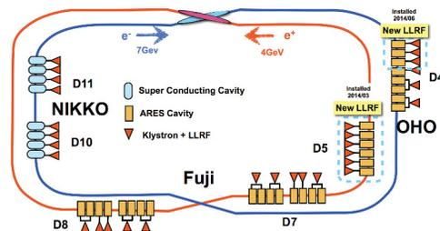
Figure 2: RF system layout for the Phase-1. Nine LLRF stations were replaced with the new ones.
