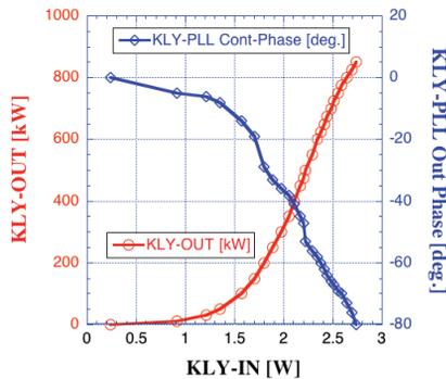
Figure 5: Klystron input-output characteristics measured under closed loop of the I/Q-FB control with the KLY-PLL control.
