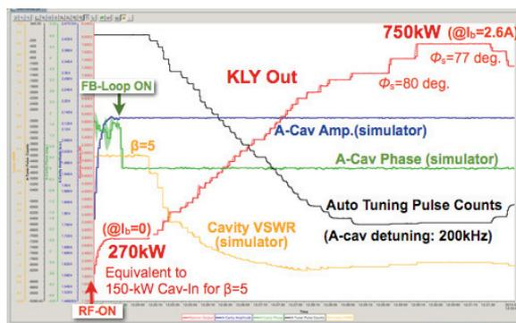
Figure 6: The chart of beam loading simulation test by using ARES cavity simulator under the closed loop for the cavity-voltage regulation control with KLY-PLL.
