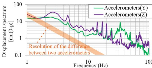
Figure 5B: Relative displacement between two points which are 10 m away along the Y and Z directions.
