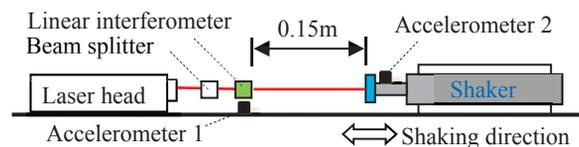
Figure 1B: Experimental system to verify accuracy using a shaker.
