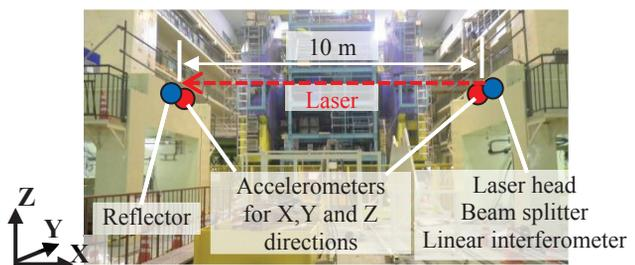
Figure 4: Measurement points around the interaction point in the SuperKEKB.
