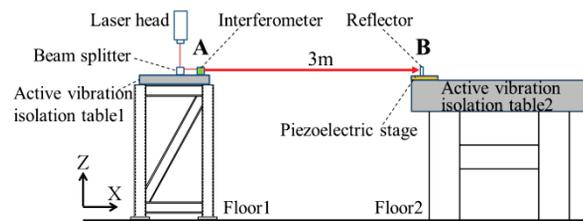
Figure 6: Experimental relative positioning control system.
