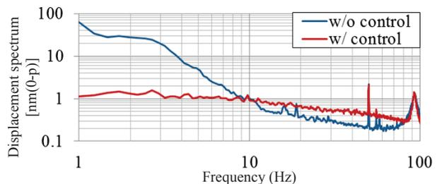
Figure 7: Relative displacement between points A and B, which are 3 m away along the X direction.
