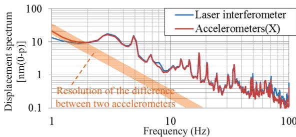
Figure 5A: Relative displacement between two points which are 10 m away along the X direction.
