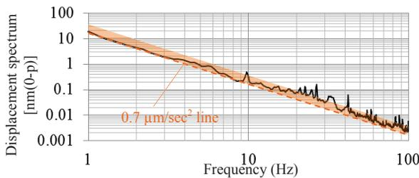
Figure 2: Relative displacement spectrum evaluated by the difference between the two accelerometers.
