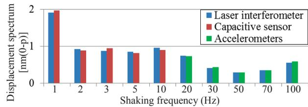
Figure 3: The smallest measurable relative displacement compared with the capacitive sensor or accelerometers.
