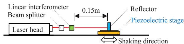
Figure 1A: Experimental system to verify accuracy using a piezoelectric stage.
