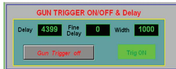
Figure 3: Operating interface of electron gun trigger.
