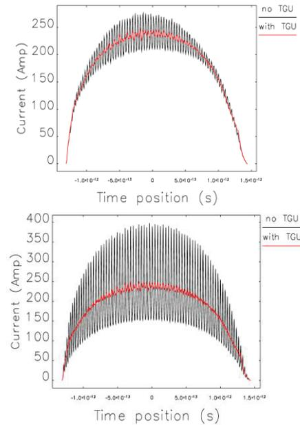
Figure 2: (Color) Longitudinal beam current profiles with (red) and without (blue) TGU at BC exit. Top: with initial current modulation; bottom: with initial energy modulation.
