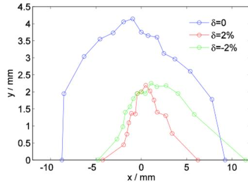
Figure 2: Dynamic apertures of the SSRF-U storage ring.
