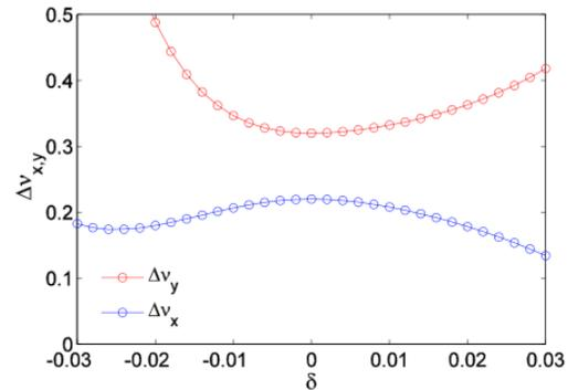
Figure 3: The tune shift with the energy deviations.
